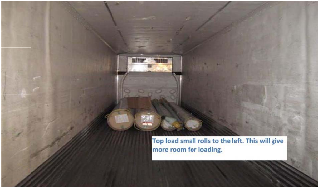
Actual dimensions are 12' feet long. Once small roles are top loaded to the left, palletized freight can be loaded on right hand side. Cube as 144L x 48W x 96H
